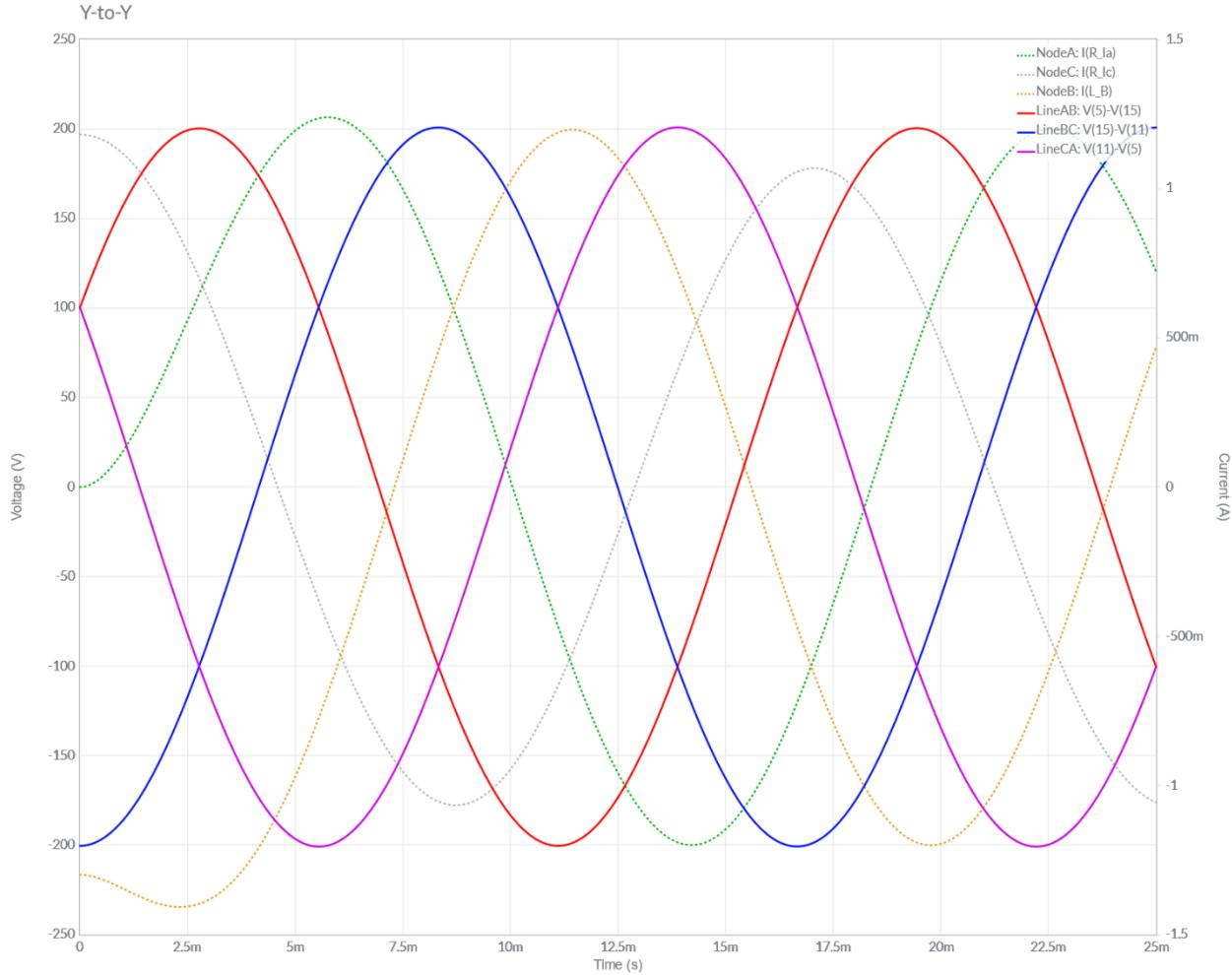
The variation from the default circuit is even less pronounced than Part Four: The line voltages of BC and CA only vary by  $\sim 0.5$  V this time, and the C line current has new peaks at  $\pm 1.068$  A.
