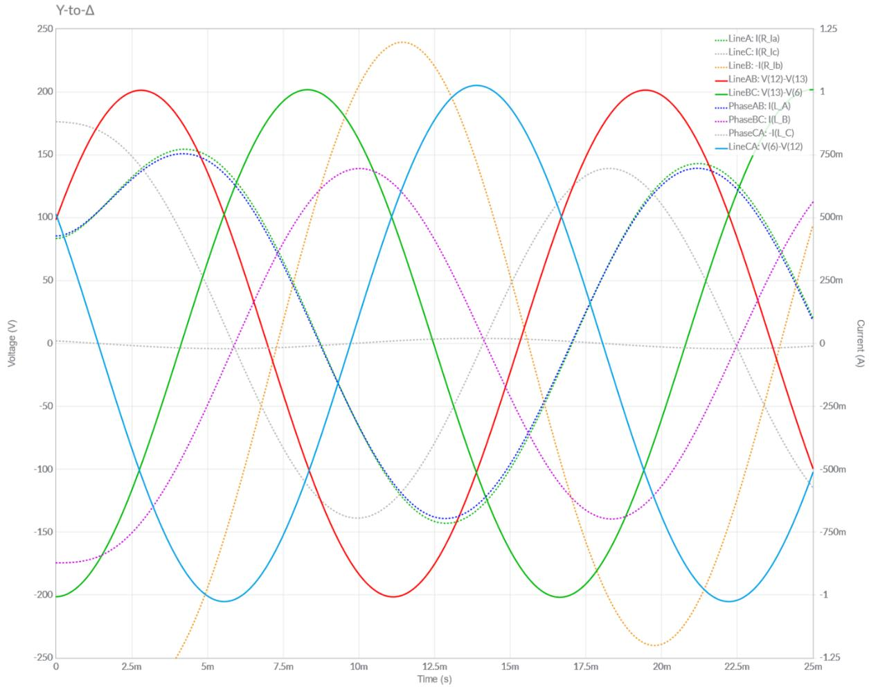
In this case, the voltages all throughout had minimal change, with the CA line having the largest difference from the default at  $\pm 205.17\text{ V}$ . The current, however, is all over the place, and to put it succinctly here is difficult.
