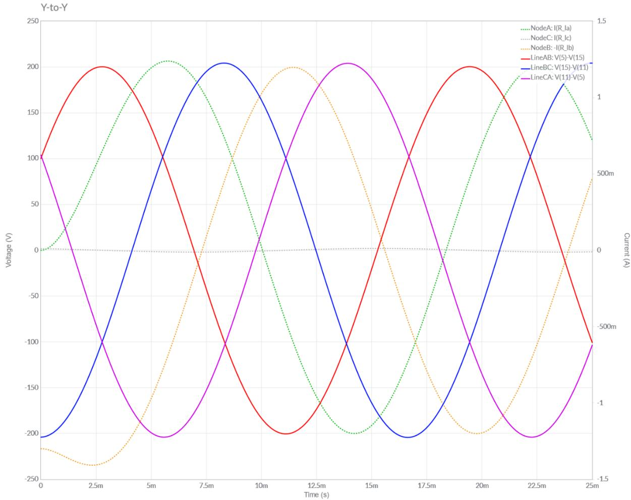
Here, the differences between the line voltages are less pronounced, BC and CA only changing by  $\sim 0.85$  V compared to default, and AB remains the same again. While the A and B line currents remain at  $\pm 1.2$  A, the C line current comes down to about  $\pm 12$  mA.
