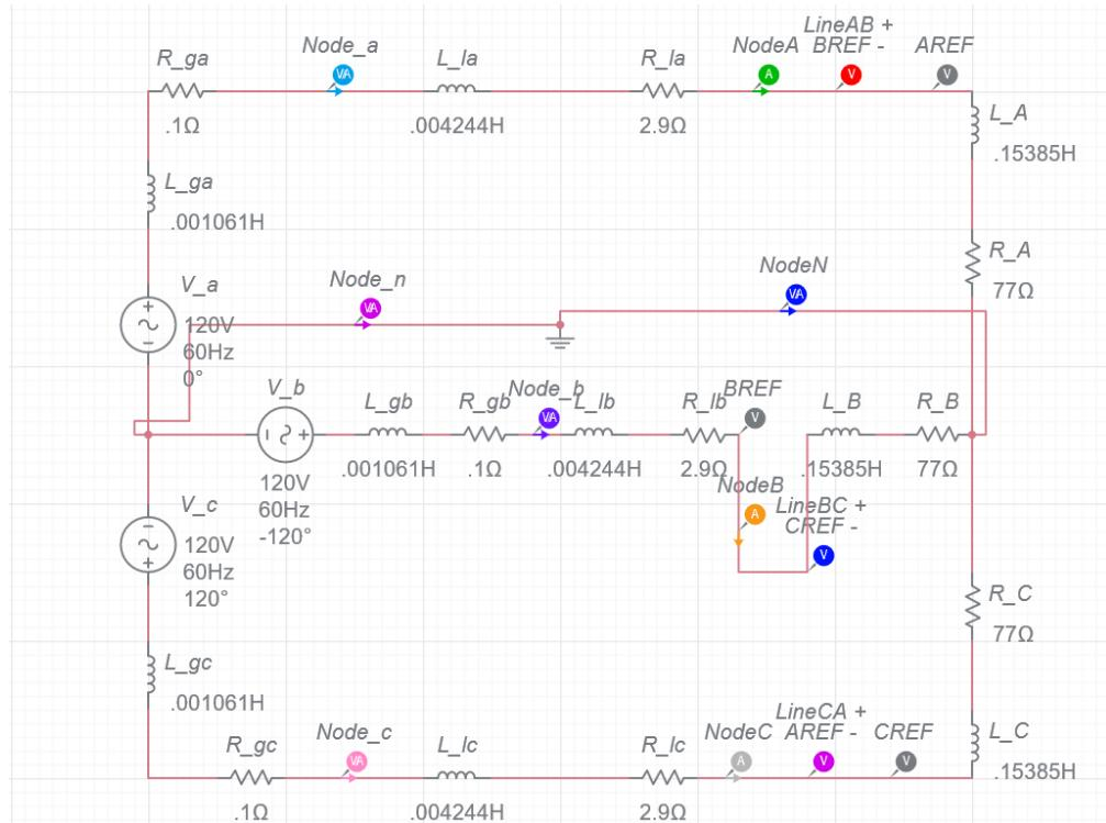
To find the voltage drop across each impedance, we must first find the total impedance followed by the current. To find the total impedance, we add each component in series and then find the RMS of the real with the imaginary portion (we will begin with just the A phase):
