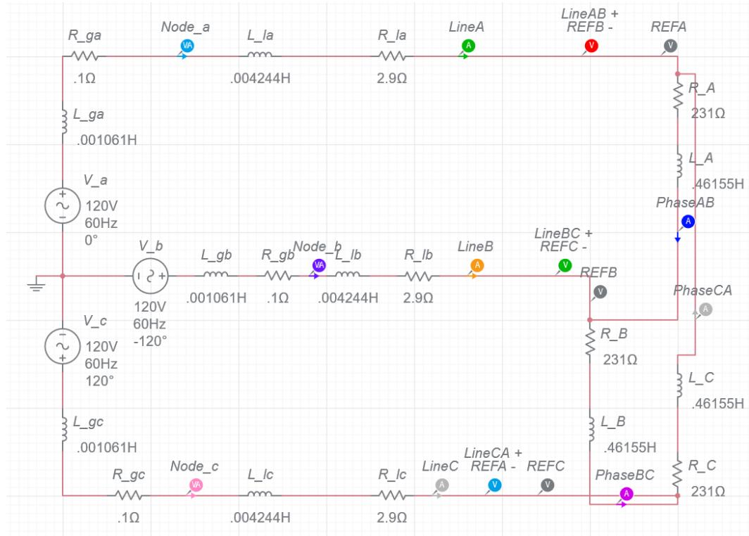
Once again, the first step in finding the voltage across each impedance is to find the values of those impedances in Ohms. Thankfully, since the calculations are done one branch at a time, as in with the Y-to-Y values in place, we can re-use the same impedance values as before:
